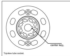
*Some tubes and tube sockets have a "center key" which must correspond! If you use "brute" force and misalign, you will damage important and expensive parts of your amplifier!!*
