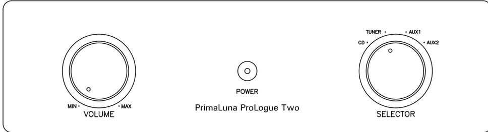
The front panel of the PrimaLuna models is made from machined aluminium, finished to match the blue metallic chassis. The volume is controlled with the knob on the left, source selection is on the right. Your sources are labelled CD, Tuner, Aux 1 and Aux 2, but all are interchangeable. There is no functional difference between the inputs. The power switch is located on the left side of the amp, just behind the front plate.
