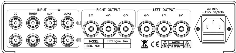
Looking at the rear panel, you will note you have four inputs and the pair of speaker terminals. Attach the positive (+) from your loudspeaker to the 4 or 8 ohm terminal that most closely matches the average impedance of your loudspeakers according to their manufacturer's specifications. The negative (-) from your loudspeaker attaches to the 0 Ohm terminal.
